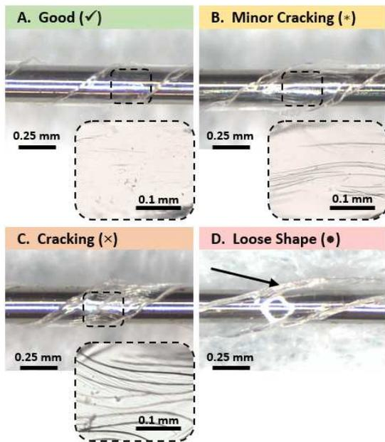
Figure 3: Examples of bare Parylene strips thermoformed into 0.25 mm helices, showing (A) a good result, (B) minor (partial-thickness) cracking, (C) cracking, and (D) loose shape, with detailed views of good and cracked Parylene.
