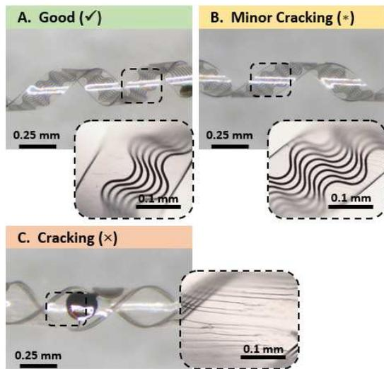
Figure 4: Examples of PMP devices thermoformed into 0.25 mm helices, showing (A) a good result, (B) minor (partial-thickness) cracking, and (C) cracking, with detailed views of good and cracked Parylene
