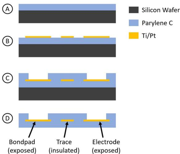
Figure 1: Fabrication process flow for Parylene-metal-Parylene devices.
