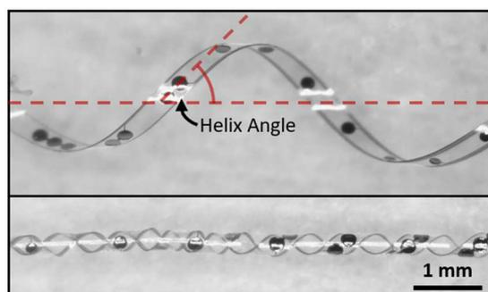
Figure 2: Photos of (top) 1.6 mm and (bottom) 0.25 mm Parylene-metal-Parylene device helices.
