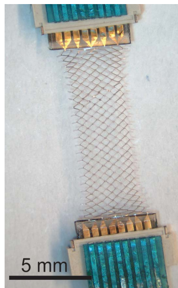
Figure 4: Devices were attached to PEEK backing and inserted into ZIF connectors during electrical testing. A stretched device is shown between the ZIF connectors.
