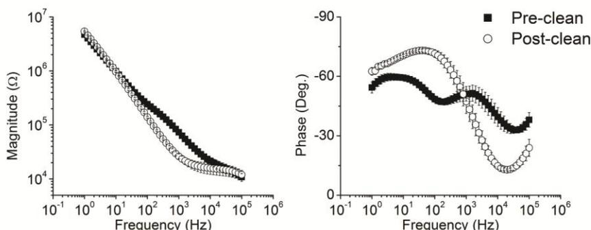
*Figure 2: Impedance magnitude and phase both before (black squares) and after (white circles) EC cleaning. Mean  $\pm$  SE, n=8 different electrodes.*
