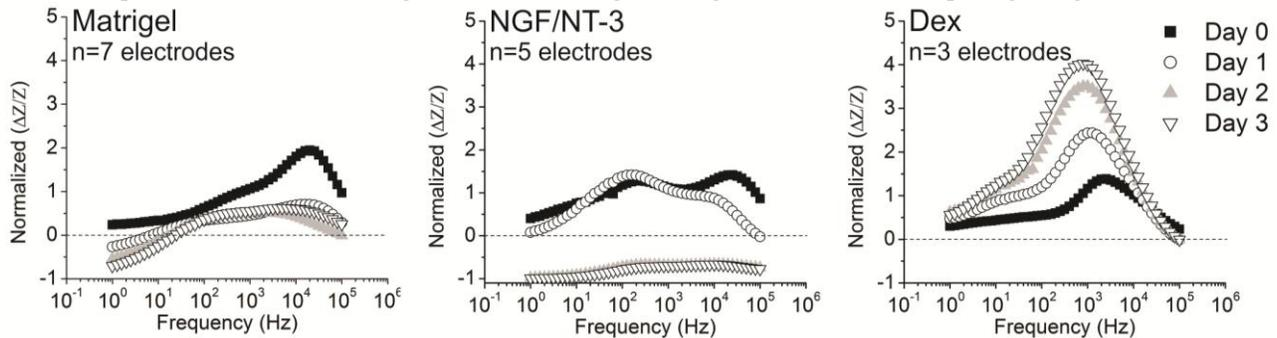
Figure 4: Normalized impedance with respect to pre-coat impedances, monitored over three days: Day 0 (black square), Day 1 (white circle), Day 2 (gray up triangle), and Day 3 (white down triangle).
