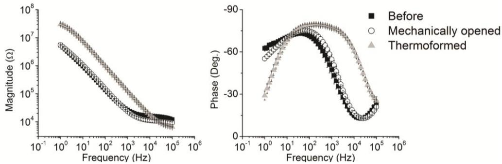
Figure 3: Impedance magnitude and phase before thermoforming process (black square), after mechanical opening of sheath (white circle) and after complete thermoforming process (gray triangle). Mean  $\pm$  SE,  $n=8$  different electrodes.
