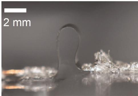
**Figure S1** Side image of a test device (700 nm serpentine trace) bent using a movable stage, while DC resistance is recorded.
