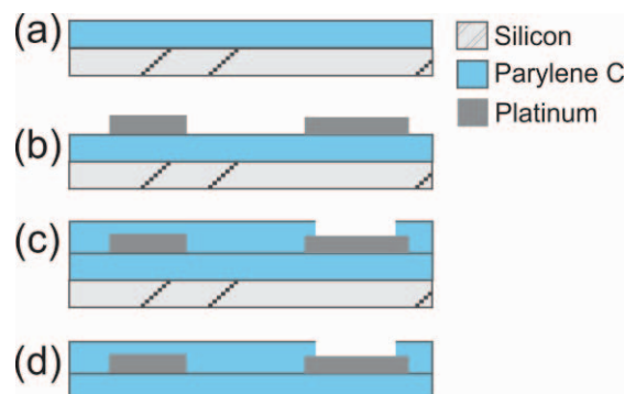
Figure 2: Flow sensor fabrication process
