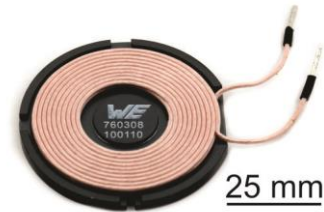
Figure 6: Primary coil with ferrite core to improve coupling with thin film (secondary) coil.
