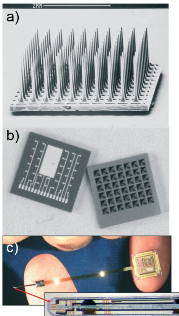
**Fig. 2** Examples of microfabricated implantable devices machined from silicon. (a) Intracortical recording electrode array: reprinted from ref. 91 © Elsevier 1998. (b) KOH etched silicon drug release microchip: reprinted from ref. 9 © Elsevier 2003. (c) Cochlear prosthesis stimulating electrode (inset) connected to application specific integrated circuit: reprinted from ref. 94 © Elsevier 2008.
