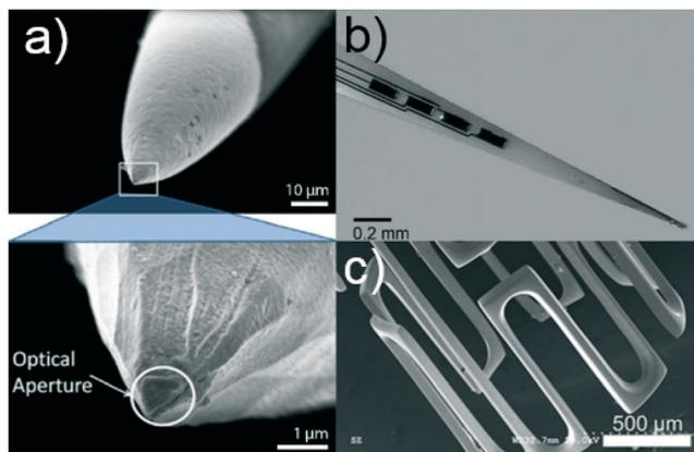
**Fig. 3** Examples of microfabricated implantable devices machined from glass, ceramic, and metal. (a) Glass fiber ‘optrode’ for optical neural stimulation: reprinted from ref. 113 © IOP Publishing 2009. (b) Ceramic shank electrode for electrochemical sensing of L-glutamate: reprinted from ref. 126 © Elsevier 2002. (c) Arterial stent fabricated from stainless steel with electro-discharge machining: reprinted from ref. 133 © Springer 2011.
