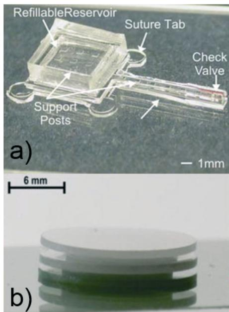
Fig. 5 Examples of microfabricated implantable devices fabricated with micro-molded polymers. (a) Refillable drug delivery device for chronic implantation, fabricated through PDMS soft-lithography: reprinted from ref. 192 © RSC Publishing 2008. (b) Microfabricated bellows cast from Parylene C onto a polyethylene glycol mold: reprinted from ref. 201 © Springer 2012.
