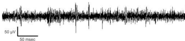
Figure 8. Representative 500 msec trace from a 300-Hz high-pass filtered electrophysiological record from thermoformed PSE at 21 days post-implantation into the rat motor cortex.
