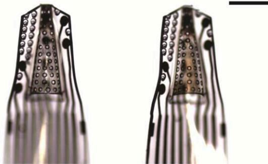
Figure 2. Optical micrograph of the tips of a 1 $\times$ 2 perforated Parylene sheath electrode array. Scale bar = 200  $\mu\text{m}$ .
