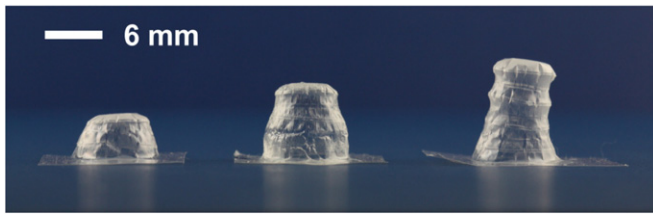
Figure 15. Photographs of bellows (6 mm ID, 9 mm OD, 0.4 mm H , 13.5 \mu\text{m} wall thickness) with 1, 2 and 3 convolutions subjected to pressure just below burst pressure and exhibiting plastic deformation.
