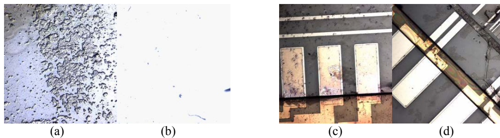
Figure 3: PC12 cells grown on PEI-coated glass coupon (a) and untreated microfluidic devices (sensor contact pads shown) (c). Same surfaces shown after cleaning (b,d). A PC12 soma is ~10 μm in diameter.
