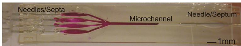
*Figure 1. Microfluidic device with integrated interconnect. Fluid is introduced into the microchannel via a needle array which pierces the septa.*
