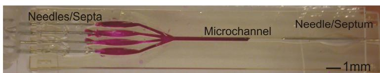
Figure 1. Microfluidic device with integrated interconnect. Fluid is introduced into the microchannel via a needle array which pierces the setpa.
