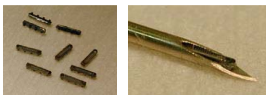
Figure 2. Microfabricated needle-implantable IOP sensors: (left) Concept of integrated device packaging; (right) A fabricated device situated inside a 19-gauge needle.
