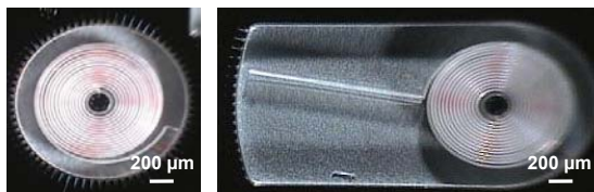
Figure 1. Microfabricated high-sensitivity parylene IOP sensors with 1.1-mm-diameter spirals.
