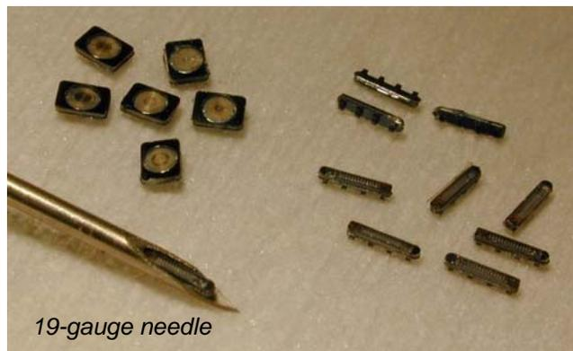
**Figure 5.** Microfabricated implantable devices.
