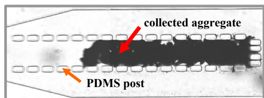
Figure 11: In-channel aggregate collector.
