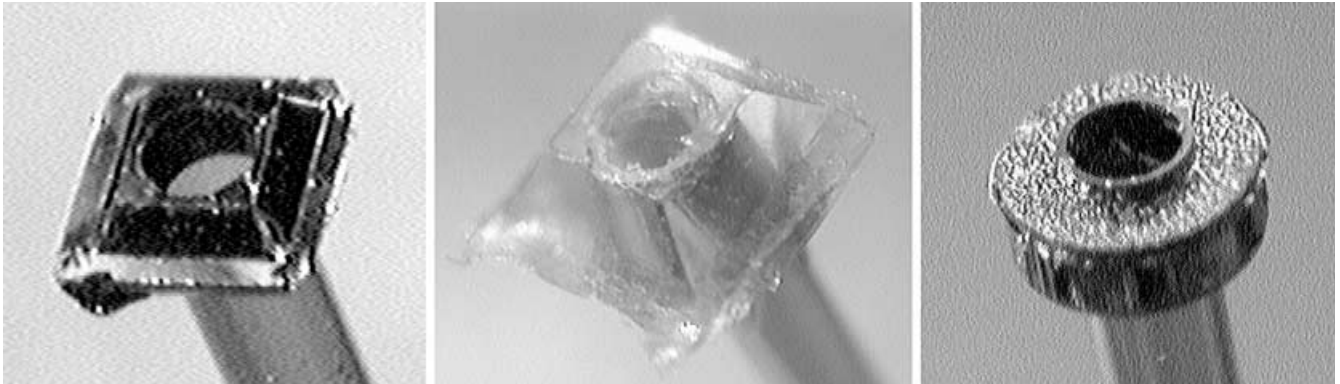
Fig.6 (a) Bulk, (b) molded, and (c) post couplers with capillary tubing
